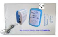
This is a bed leaving detection alarm system, part of the TumbleCare fall prevention range designed by Medpage. The bed sensor positioned under a patients bed mattress will detect their presence or exit. On exit the alarm control transmitter sends a radio alarm signal to the carer alarm station to produce an audible and flashing light notification.
